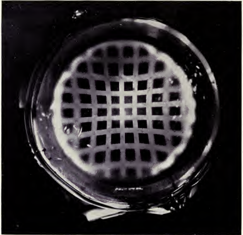
Fig. 76. Image Distortion in Uncorrected Image Tube
